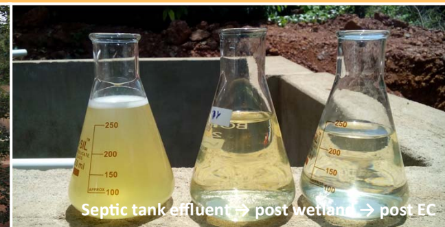
Community scale plant
